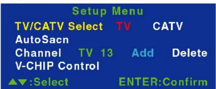
TV/CATV SELECT: To select TV signal input between off-air and cable service.
